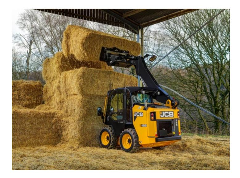
The optional electric quick hitch is fitted with a single-point lock-and-unlock flag for optimal visibility, to ensure that the attachment is safely locked and unlocked.
